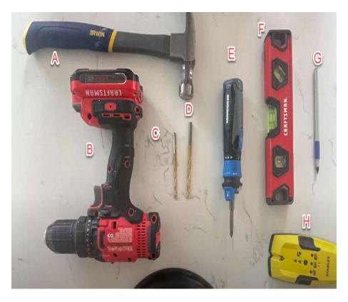
A.Hammer B.Drill C. 3/8 Inch Drill Bit D.One-quarter Inch Drill Bit E. Screwdriver with Phillips Head F. Level G.Pen H.Stud Finder
