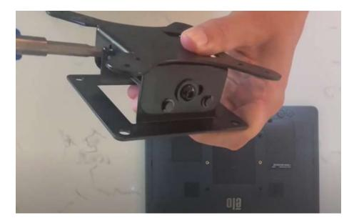
**3** Take the flat part of the mount and position it on the back of the kiosk so that it lines up with the four holes.
