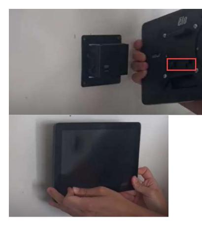
**15** Finally secure the device to the mount by adding in the screw we took out in the beginning. If you ever need to remove the device from the wall, just remove the screw.
