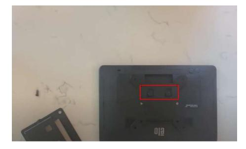
5 Then screw the four small silver screws into the holes to attach the mount to the device.
