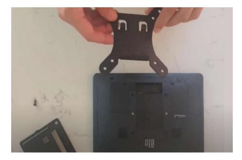
4 Make sure that the metal hooks are oriented downwards.
