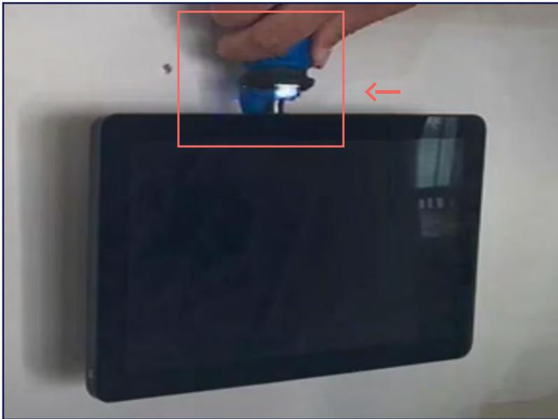
**16** If you need to change the angle of the device, you can change this by loosening, repositioning and tightening this screw on the side with the included Allen wrench.
