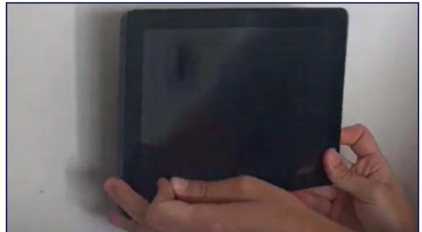
**15** Finally, secure the device to the mount by adding in the screw we took out in the beginning. If you ever need to remove the device from the wall, just remove the screw.
